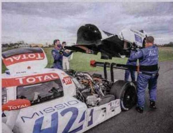
**LEFT** GreenGT will supply the battery, engine and transmission for the hydrogen cars. The fuel cell, power control hardware and software, compressors, and cooling system will be open to development by the teams
