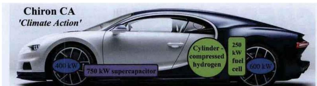
**1,000 kW, only 1,600 kg, 170 mph continuous cruise, 60 to 180 mph in 10 secs**
