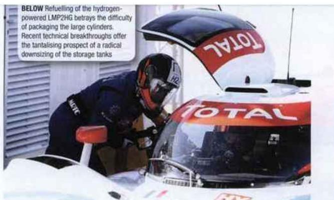
**BELOW** Refuelling of the hydrogen-powered LMP2HG betrays the difficulty of packaging the large cylinders. Recent technical breakthroughs offer the tantalising prospect of a radical downsizing of the storage tanks
